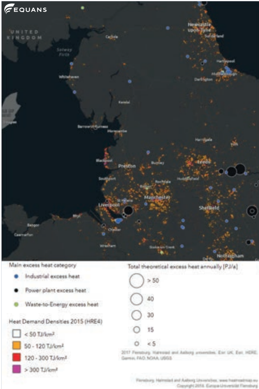
Figure 31 Heat demand density and excess heat from industrial sector in North West
