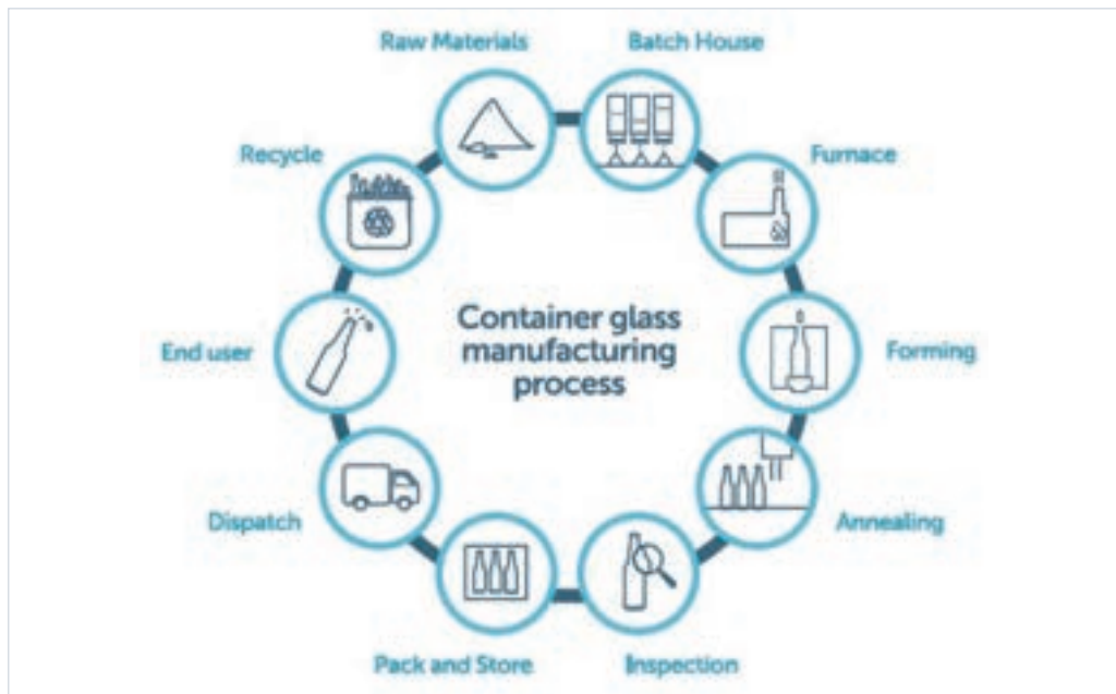
Figure 88 Container glass manufacturing process (96)
